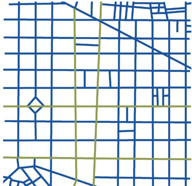
Barcelona Grid based Cerda's 1859 plan for the expansion of Barcelona Square block (113 metres wide) structure of the grid gives equal priority to north - south and east-west movement.
