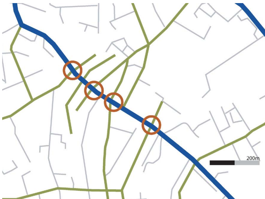
Ranelagh Village Dublin Signal controlled pedestrian crossings located at 80-150 metre intervals
